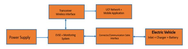
Electric Vehicle Supply Equipment (EVSE) System
